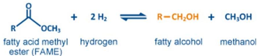
This methanol produced by the hydrogenolysis reaction is recycled back to the esterification stage to minimize the requirement for methanol make-up.
