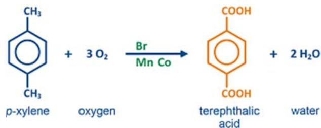
The CTA is largely insoluble, and consequently the reactors contain significant amounts of solid product crystals. The main impurity of the CTA relative to PTA is determined by the 4-carboxy benzaldehyde (4-CBA) content.
